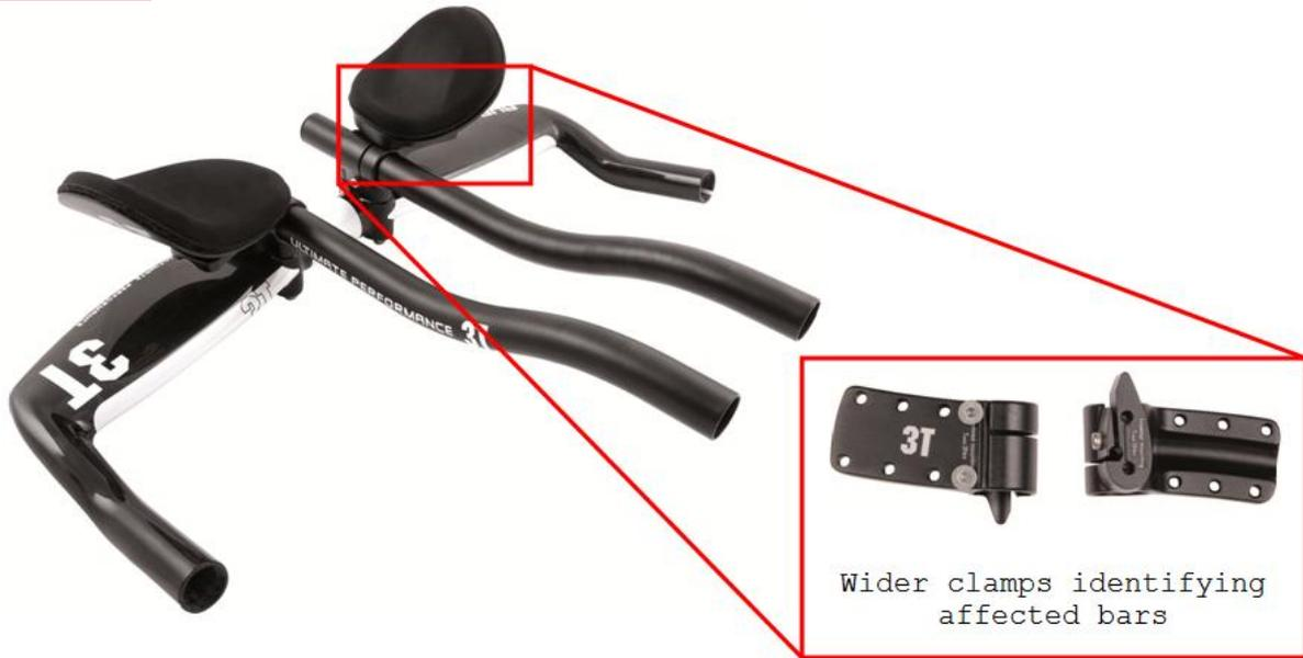
Figure 1: wider clamps on an Aura PRO aerobar
